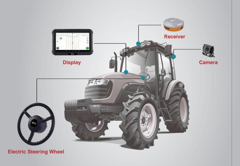
The eSteer 10 system features an all-in-one controller that integrates a 4G module, IMU sensor and GNSS module, making it easy to install and transfer between vehicles. No additional wheel angle sensor is required for the eSteer 10, further enhancing its ease of installation.
